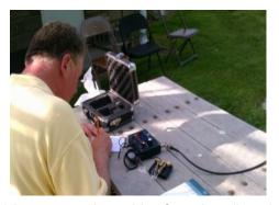
The club's new Kenwood TS-590 is set up and capable of running all modes. Setting up the 590 for computer rig control and digital modes is very easy since only one USB cable from the radio to the computer is necessary.
