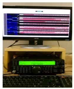
The filtering on the 590 is also very good and easy to use for digital modes. Below is a photo of the digital program DM780 decoding RTTY-45 with the TS-590 filter set for about 500hz.
