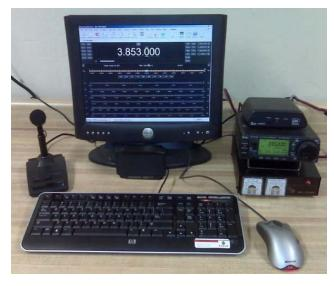
FlexRadio Systems Flex-5000A Dual Receivers Internal Auto Tuner Power SDR v2.0.16 (Beta) Woodbox Tmate (CAT/VFO) Bencher Paddles AL-80A Amplifier Palstar AT4K Tuner Heil Pro Set Quiet Phone
