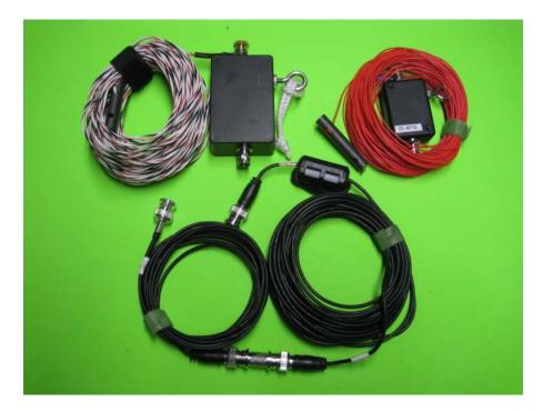
I mostly focused on a HWEF40 since the two most popular bands that I use when I set up portable are 20 and 40 meters. If all you need is 20 meters, make your's only 32 feet 6 inches long. If you would like to include 80 meters, the wire cut length will now be 131 feet long. A HWEF80 will cover 15, 17, 20, 40 and 80 meters. You can use it on 10 meters but the SWR will above 2 to 1. The HWEF80 is in fact resonant on 10 meters, but it does have an elevated SWR.
