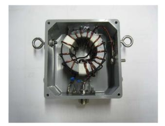
Shown below are two HWEF40 meter antennas. The one on the right shows an UnUn rated for 25 watts and the antenna wire is #22 teflon insulated wire, 65 feet 6 inches in length. The core used to make this UnUn is an FT 82-43. It is a 64 to 1 UnUn and #22 enamel wire was used on the core. I wanted a HWEF that would fit in my shirt pocket, hence the reason for the #22 teflon wire and the UnUn rated for only 25 watts.
