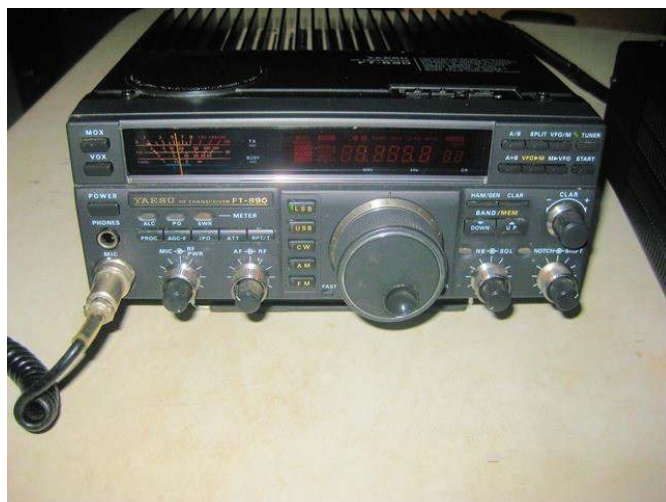
Yaesu FT-890 Transceiver with built-in Automatic Tuner 160 through 10 meters, 100 watts
