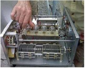
**George / N3SQD** acquired a legal limit home brew antenna tuner for show and tell. The workmanship is amazing A view of the inside of the tuner. The light bulbs serve as the 100w dummy load. George will need this tuner when he brings his BTI amp online.
