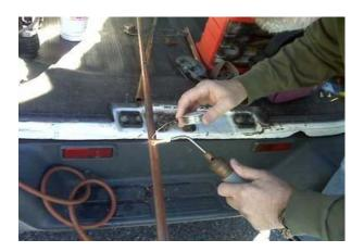
**Bob / NE2C** built a mobile antenna with masts and coils for 80, 40, and 20 meters. The engineering is very clever and the build quality is impressive. The "Joints" of the support assembly "pivot" so the trunk can be opened without disconnecting the antenna support.
