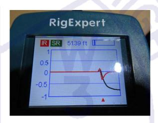
Programming the antenna analyzer is super easy. The one setting on the analyzer that is important to make, for accurate readings, is to program the velocity factor of you coax. If you do not know it, run the TDR anyway. It will show a fault if there is one, but the point of failure will just be an estimate. It will get you to the general area of the failure.
