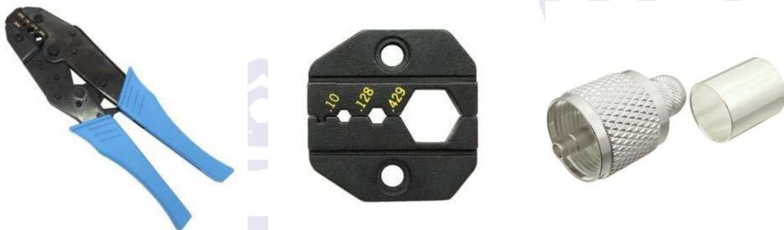
Coaxial cable like some LMR 400 and 9913 coax use a solid center conductor. Here lies a problem but it is correctable. Once you attach the connector to the coax and crimp the shield, you can also crimp the center pin to the solid center conductor. Once completed, you must solder the center pin to the center conductor. This is an acceptable practice.
