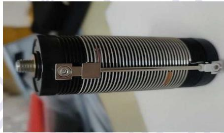
The contact slider is extremely easy to slide up and down, by hand, for changing bands. Look closely at the fourth turn on the coil from the left hand side of the assembly. It is colored brown. That shows you where the tap is to be place
