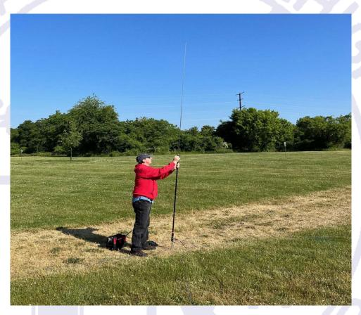
Adjusting the contact slider on the coil. The antenna was erected at Franko Park.
