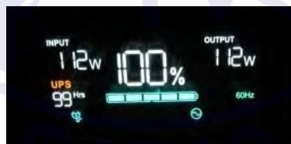
The bottom left corner of the display shows the power station is in the UPS mode. A few items in the radio shack are on line showing its load on the power grid is 112 watts.
